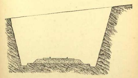
Fig. 6. EXCAVATION IN BOCK.
